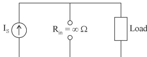
For the ideal current source, the current is completely independent of voltage source and has infinite internal resistance.
