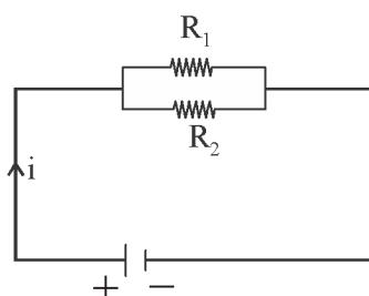
$$R_{eq} = \frac{R_1 R_2}{R_1 + R_2} \quad \text{Parallel connection}$$
