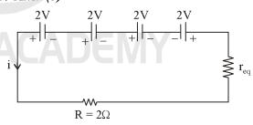
each cell has  $0.5 \Omega$  internal resistance
